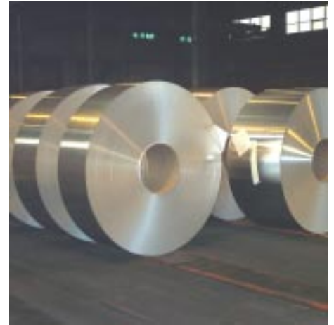
Jupiter Aluminium melts scrap metal and forms it into custom specified coiled sheets.
